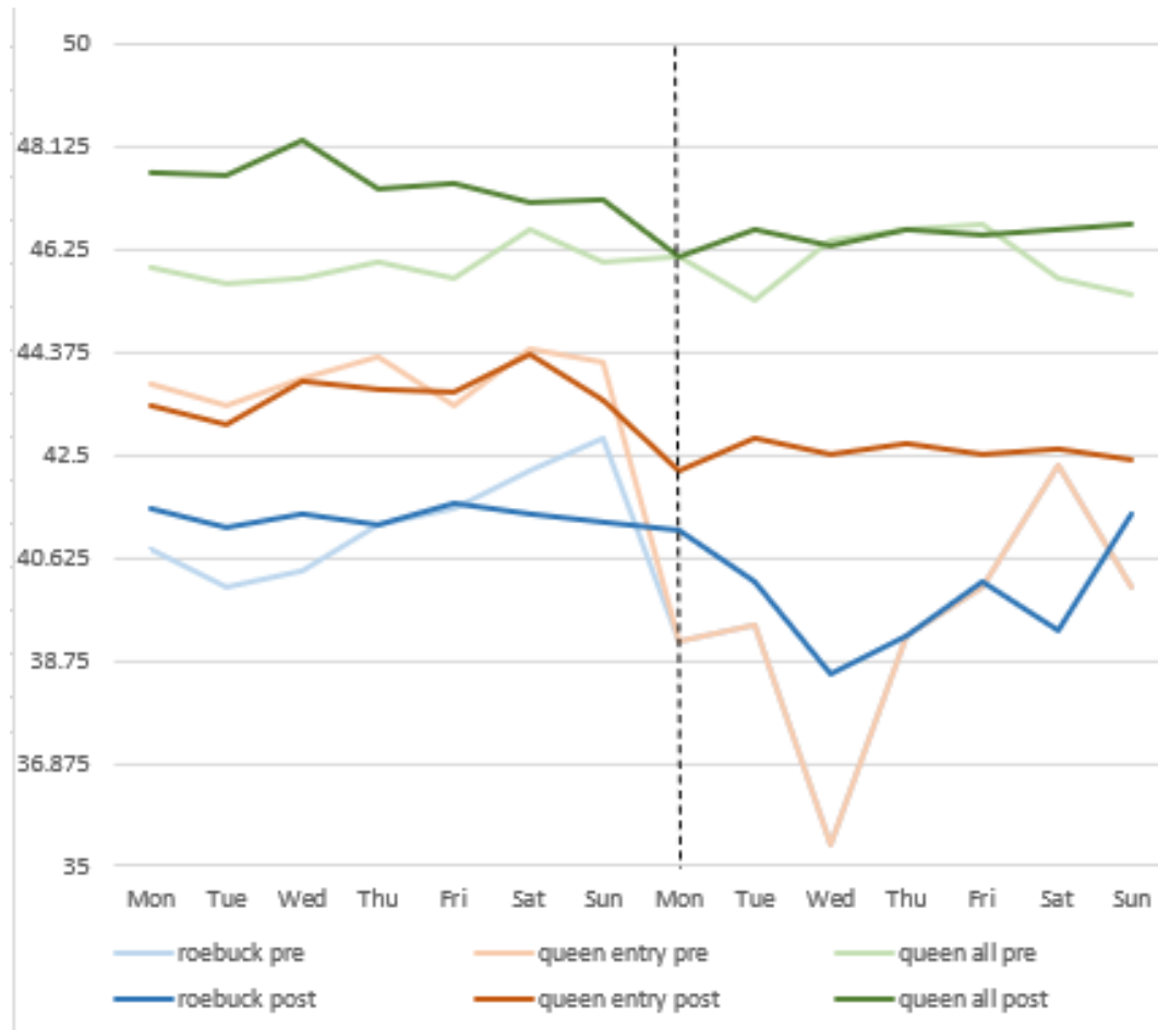
Average pre-signage and post-signage speeds by day in the three Westport area sites.
